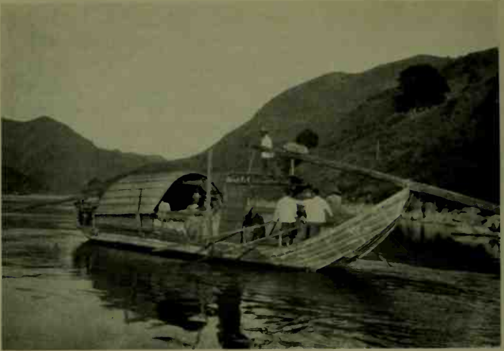
The Fukien Min is so swift that on the larger cargo-boats the steersman is put high up on a platform and his mighty oar-rudder is weighted with a stone or a part of the cargo
